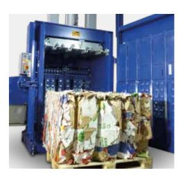
Hydraulical bale ejection
