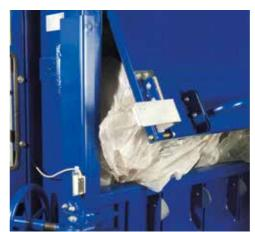
QuickDoor® The swinging-sliding door with an automatic opening ensures a fast and safe filling of the press chamber.
