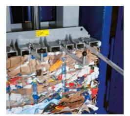
Integrated strap- and wire hooks In the press plate integrated strap- and wire hooks ensure an easy, comfortable and fast bale tying.
